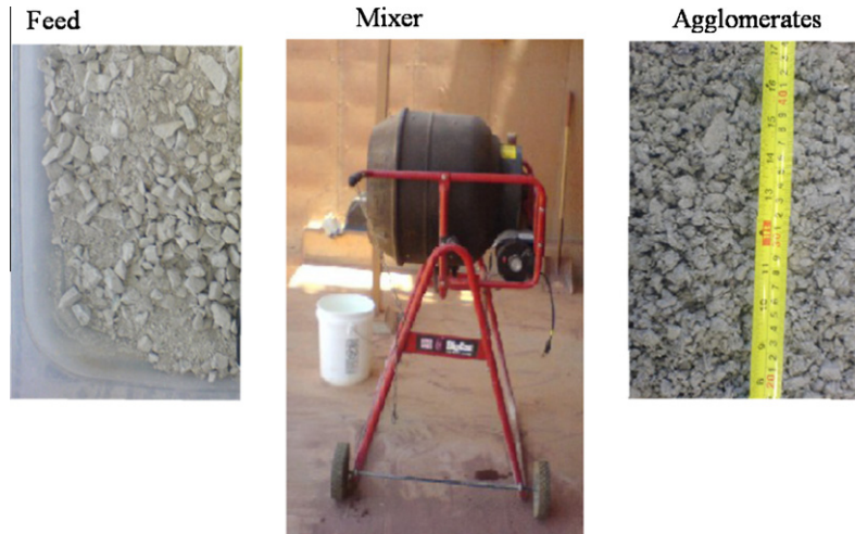
Fig. 2. Feed, plastic drum cement mixer, agglomerates.
