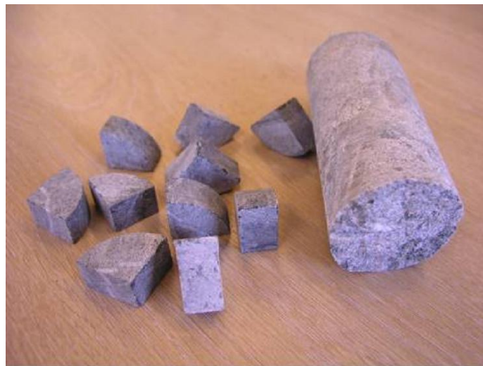
Figure 2 - Particles Selected for SMC Testing from Cutting Drill Core
