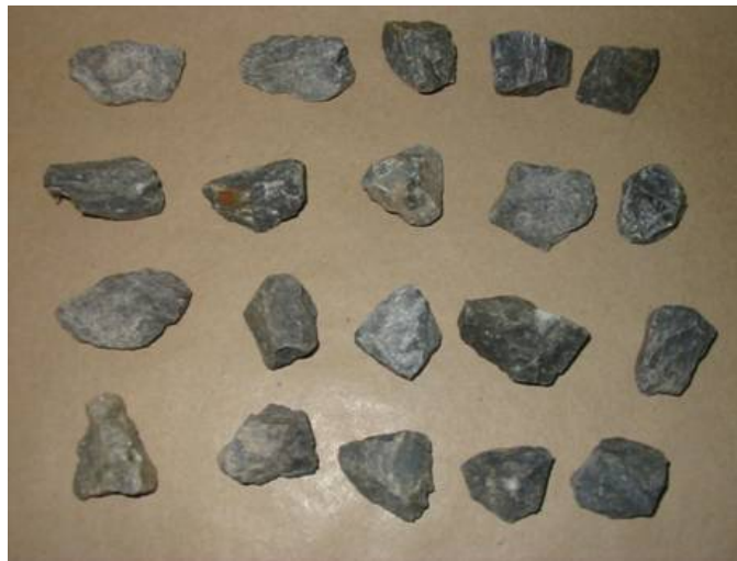
Figure 1 – Particles Selected for SMC Testing from Crushed Rock
