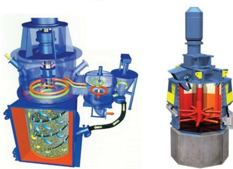
Figure 2.8 Left: Vertimill ® ; right: stirred media detritor (Lichter & Davey, 2006)
