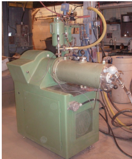
Figure 3.10 M20 stirred mill installed at UBC
