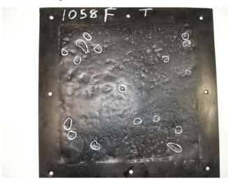
Photo 2: 1.5mm HDPE tested for puncture at 21°C.
