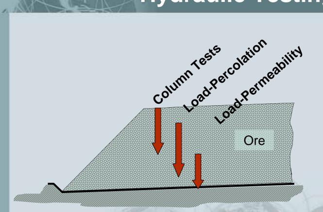
Tests simulate varying hydraulic conditions within heap
