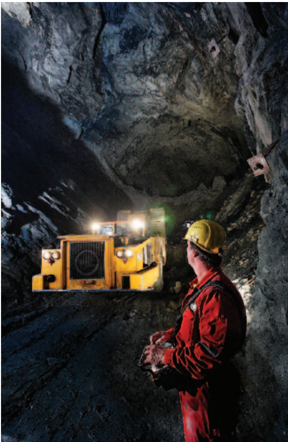
Figures 19 - 20: Sublevel stoping: left mucking of a sublevel stope by remote-controlled scooptram in the Mittersill mine, Austria; above a sketch depicting the set-up of large-scale open stoping using draw-point, from SMITH M (Ed) [2008]
