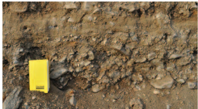
Figure 49 - 50: Alluvial mining: Artisanal panning concentrate of subrounded wolframite "gravel" from fossil placer at the Gifurwe deposit, Rwanda (top). Gravel deposit at Zakamensk, Burjatia, Russian Federation: Wolframite is contained in the sand fraction of the gravel beds in a valley downstream of the primary deposit (bottom).
