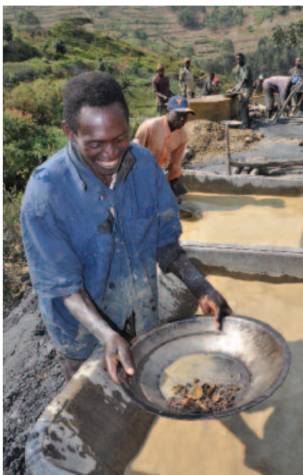
Figures 33- 35: Artisanal methods: from left to right: traditional panning of alluvial wolframite; manual jig and wooden sluice leading to corduroy sluice (downstream of a ground sluice); both at the Gifurwe mine, Rwanda. Wooden sluice boxes designed to minimise water consumption at an artisanal site in Bolivia.
