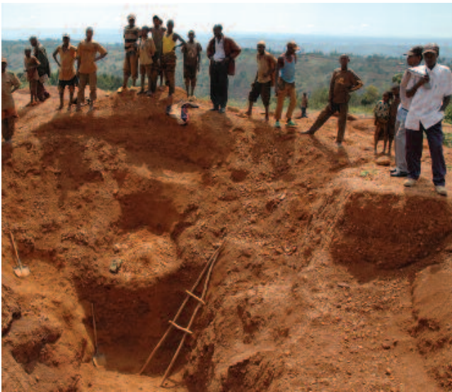
Figure 48: Artisanal tungsten mining in lateritic alteration above primary vein-type mineralisation, Burundi.
