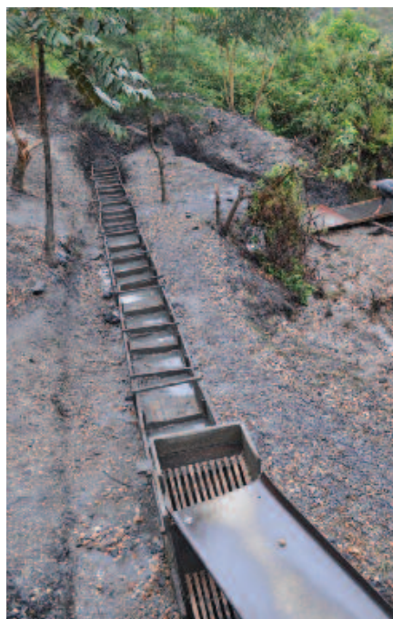
Figures 33- 35: Artisanal methods: from left to right: traditional panning of alluvial wolframite; manual jig and wooden sluice leading to corduroy sluice (downstream of a ground sluice); both at the Gifurwe mine, Rwanda. Wooden sluice boxes designed to minimise water consumption at an artisanal site in Bolivia.
