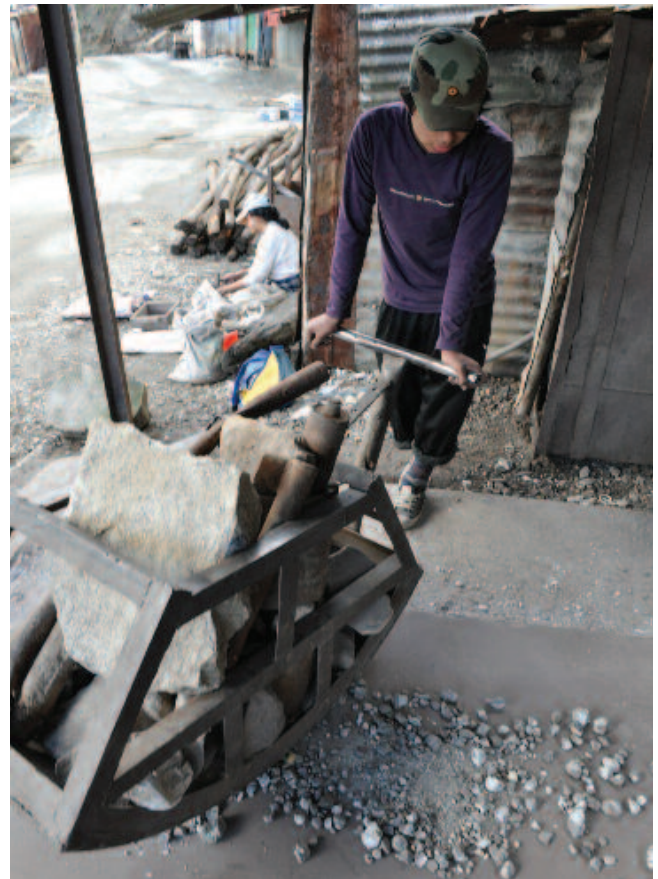
Figure 28: Secondary crushing to grinding in an artisanal operation in Bolivia, using a so-called quimbaete.
