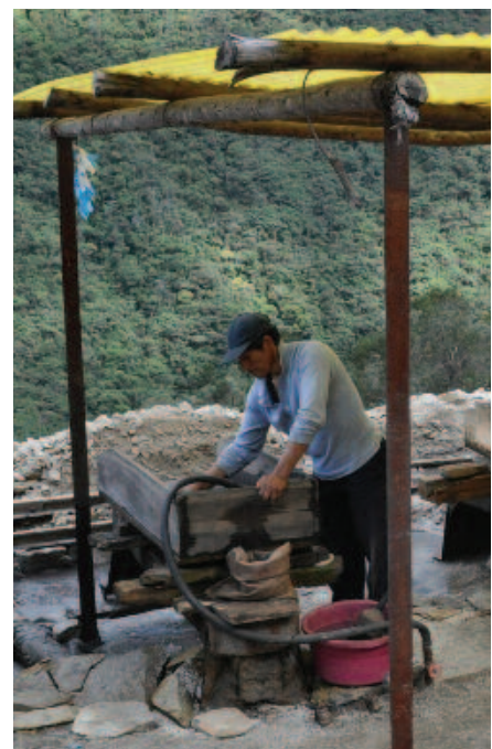
Figures 33- 35: Artisanal methods: from left to right: traditional panning of alluvial wolframite; manual jig and wooden sluice leading to corduroy sluice (downstream of a ground sluice); both at the Gifurwe mine, Rwanda. Wooden sluice boxes designed to minimise water consumption at an artisanal site in Bolivia.
