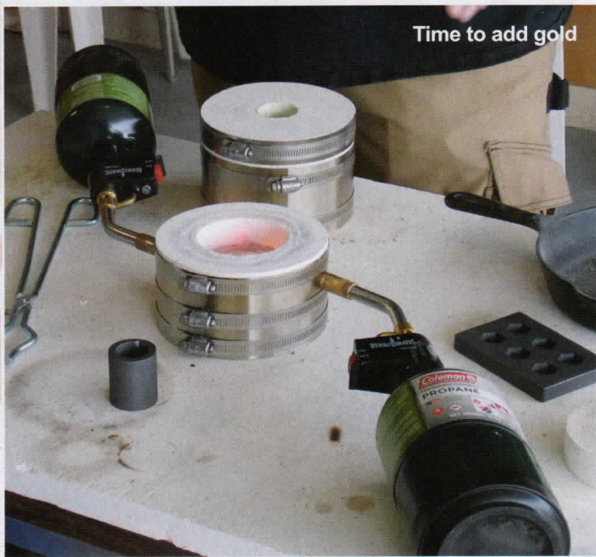
Heating the mold is a crucial step in proper pours
