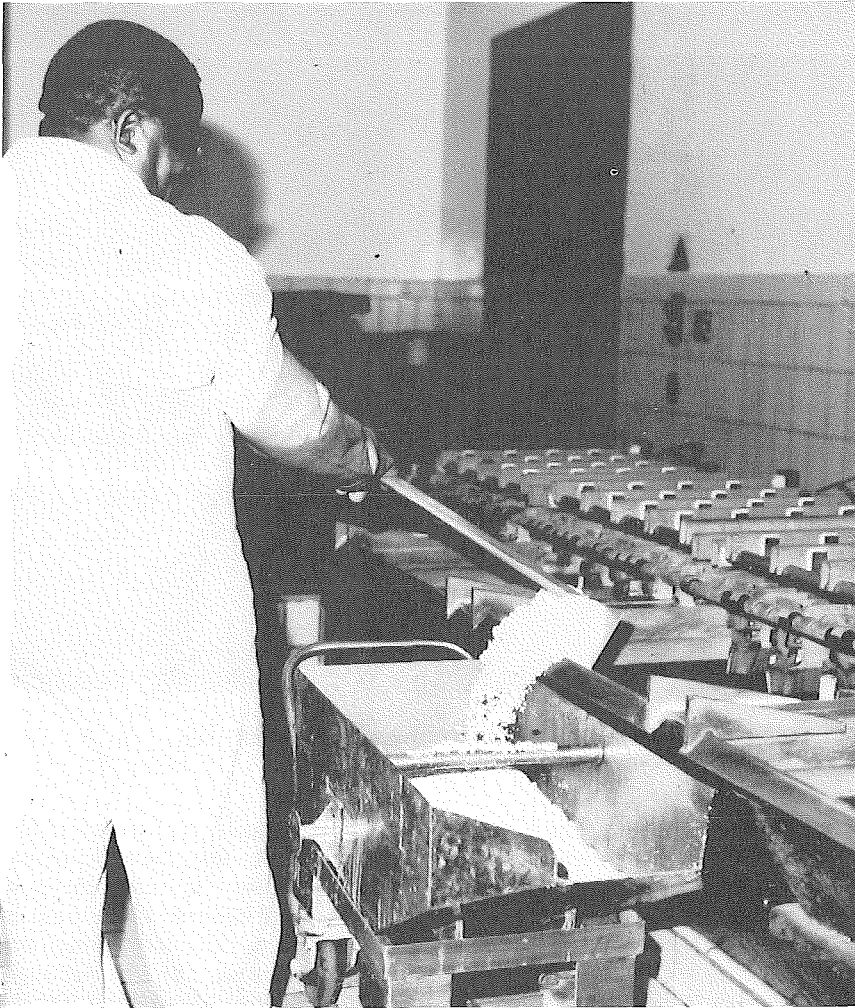
Figure 10.14. Removing silver crystals from vertical (Moebius) cells.
