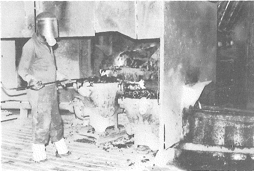
Figure 10.25. Blast furnace slag and matte stream.
