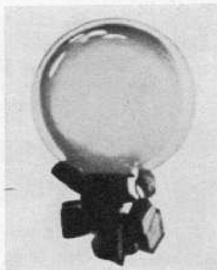
Fig. 6. Photomicrograph of galena particles in ethyl xanthate solution clinging to a small air bubble, which in turn is suspended from a larger air bubble 1 mm. in diameter. (After H. Rush Spedden)
