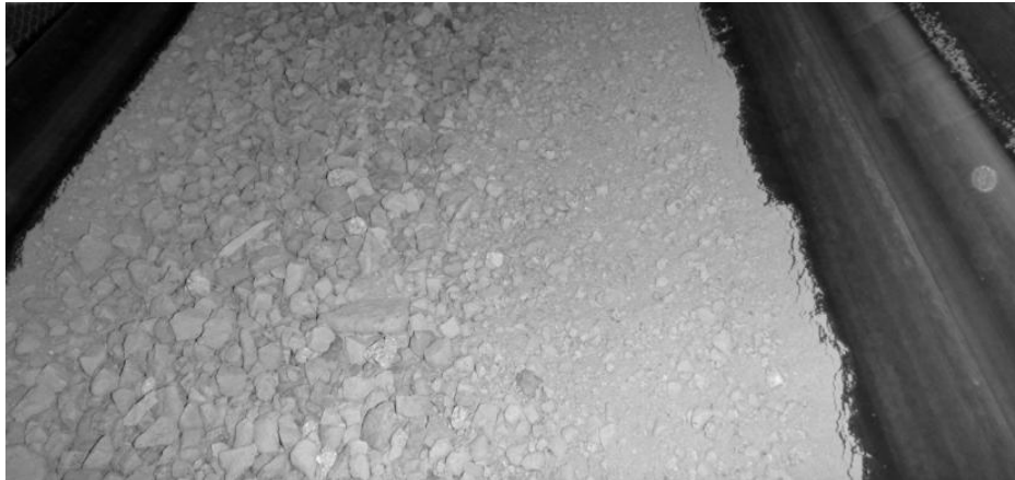
Figure 13. Feed Size Segregation on a conveyor belt.
