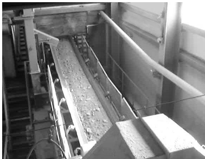
Figure 10. Flakes in the HPGR Discharge at Vasilkovka
