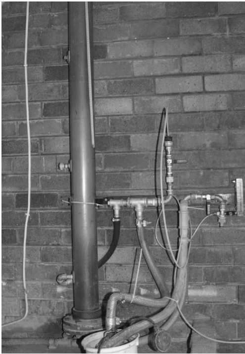
Figure 1: Modified Bikerman test rig. Used to test froth characteristics and is a tool to design and select a frother for a specific application.
