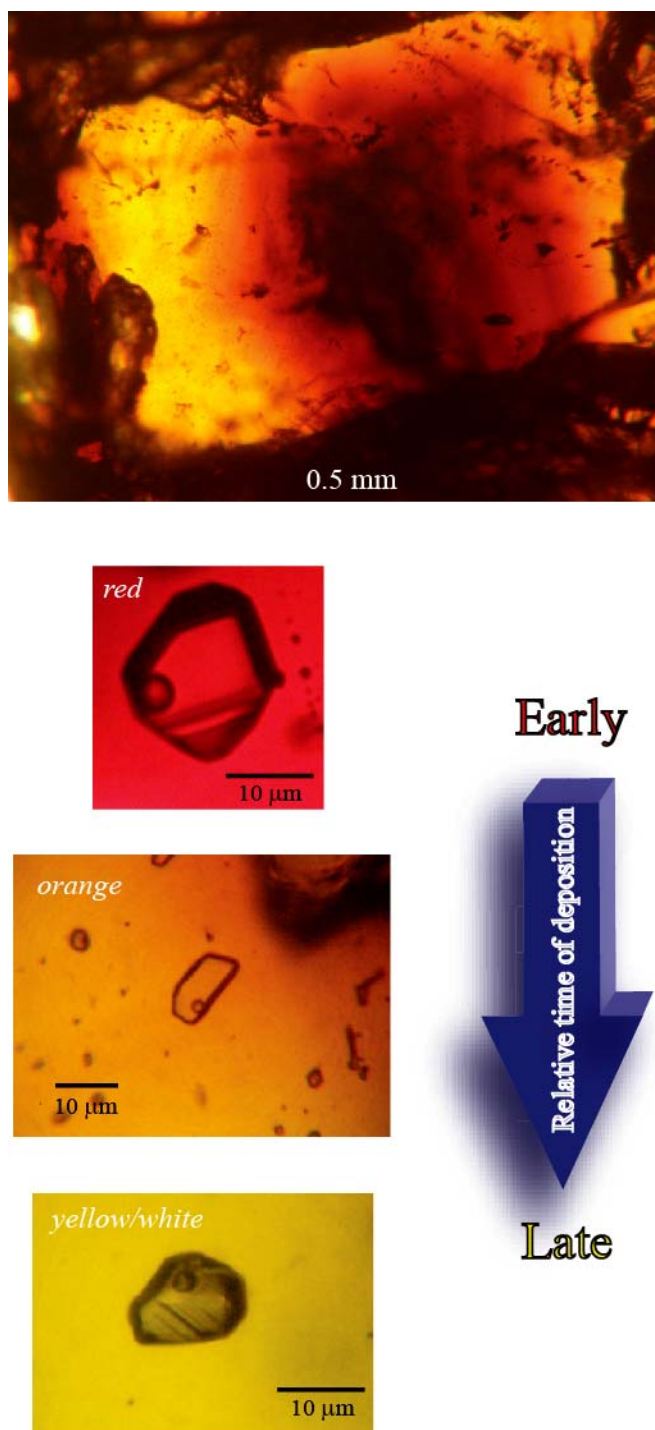
Figure 8. The upper photo shows a zoned sphalerite crystal from Ersmarksberget. The lower three photos show representative aqueous fluid inclusions in the dark red core, the intermediate orange zone and the yellow margin. The arrow indicates the relative time of deposition and decreasing salinity.
