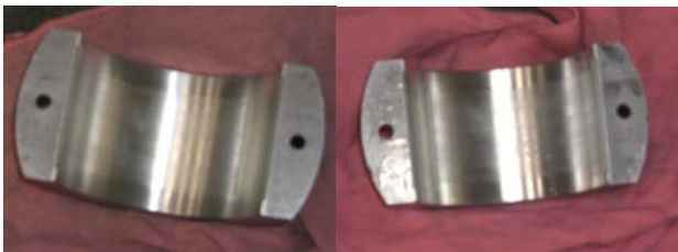
Figure 5. Post-Test Inspection of Hydrodynamic Bearings
