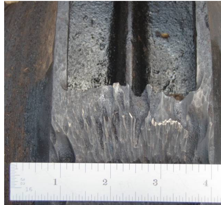
25 Chrome iron impeller tip wear
