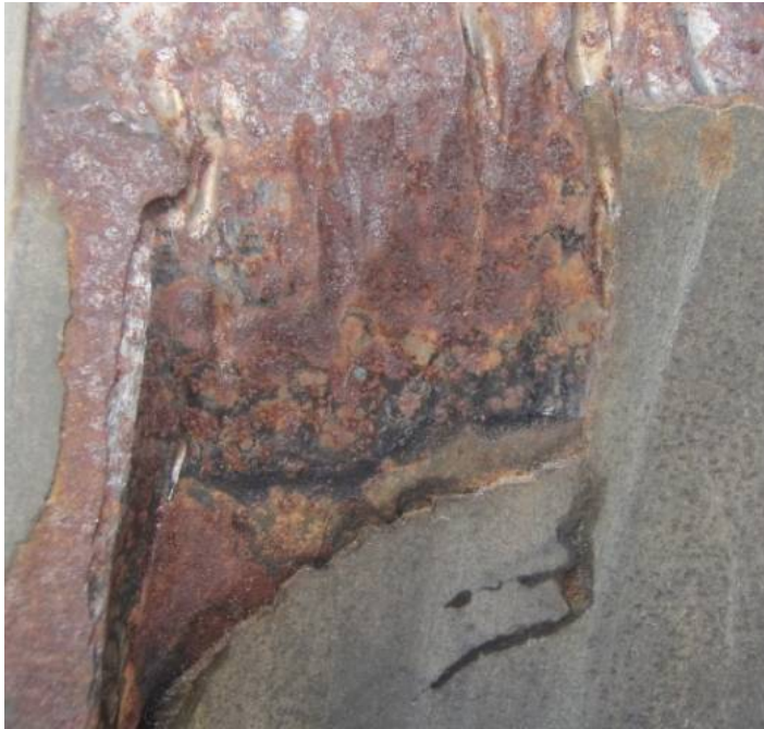
Boron Diffusion worn through (wear plate closeup)
