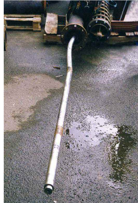
Figure 13. Pump Shaft from Pump A. (Shaft was bent after the shaft seized. The motor tripped on high amps.)
