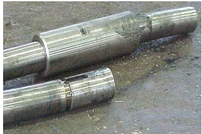
Figure 14. Damaged Pump Shaft Cut into Pieces to Remove Impellers.
