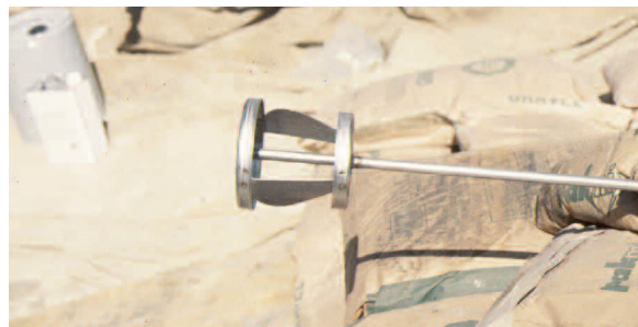
Figure 22. Mixing Blade of a Jiffy Mixer.
