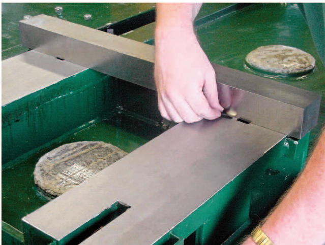
Figure 10. Measuring Flatness with Ground Bar and Feeler Gauge.
