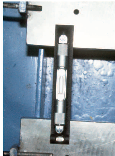
Figure 12. Level Baseplate in Transverse Direction Next.
