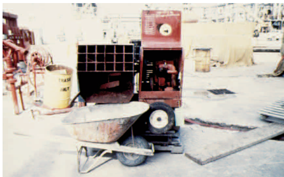
Figure 21. Typical Motorized Mortar Mixer.
