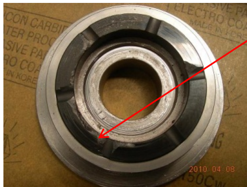
Thrust Bearing Damage
