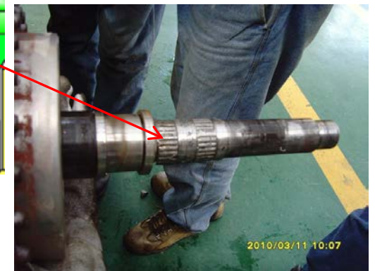
Tolerance Ring Damage
