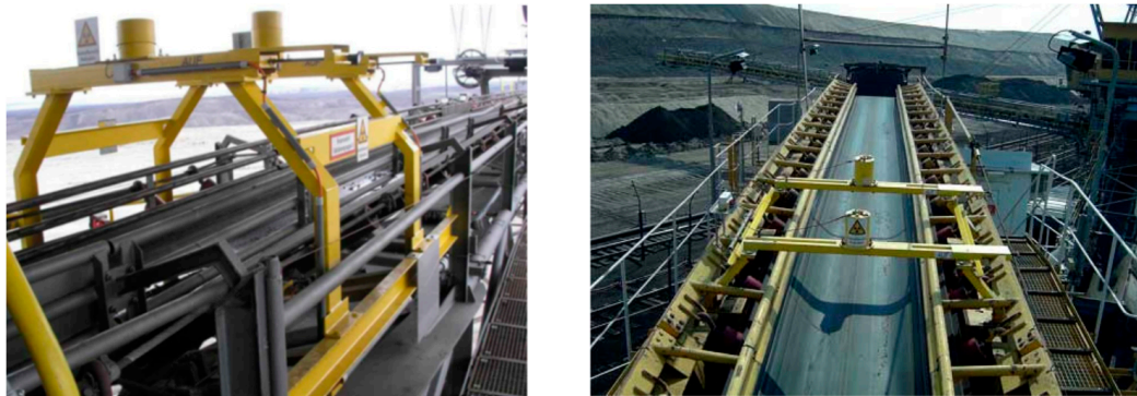
Figure 1. Radiometric sensor measurement of coal in the Profen mine (photo of MIBRAG).
