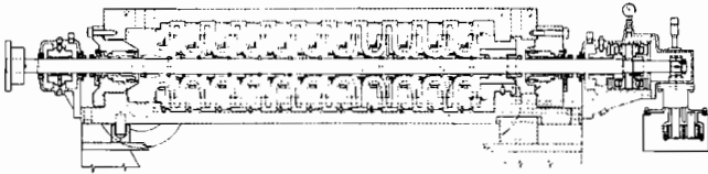
Figure 4. Safety Injection Pump.
