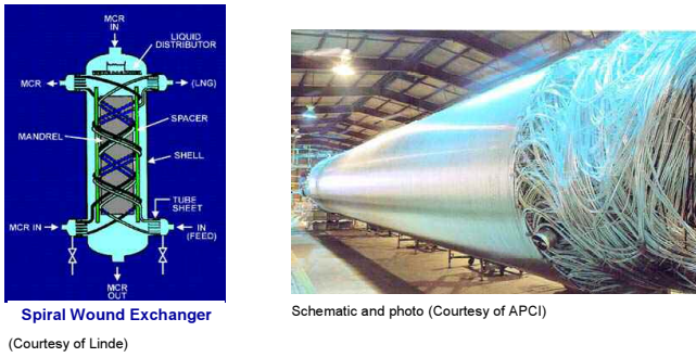
Figure 5. Sketch and Photo of a Spiral Wound Heat Exchanger (SWHE).
