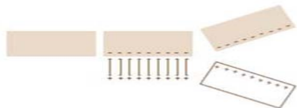
Figure 5: Electro-static charging of two separating surfaces
