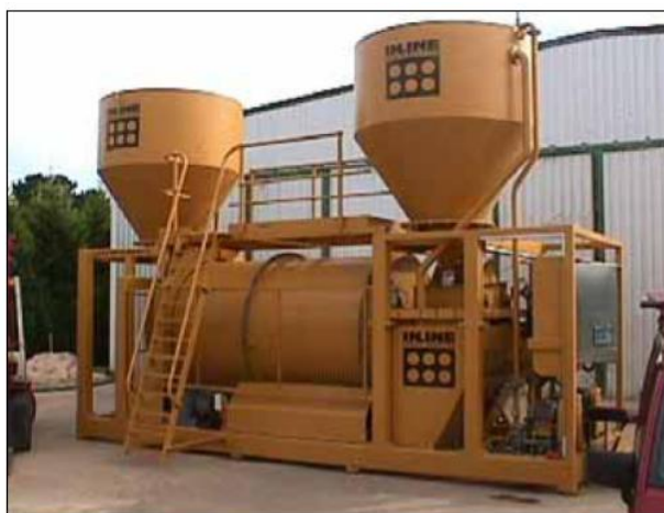
Figure 33 InLine Leach Reactor, model ILR 2000 (Gray, 2000).
