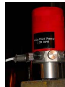
Figure 6. Battery Powered Transmitter with Pulse Input for Pump Rotational Speed.
