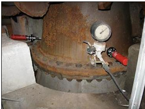
Figure 11. Pressure Instruments Around Suction Nozzle Spaced 90 Degrees Apart.
