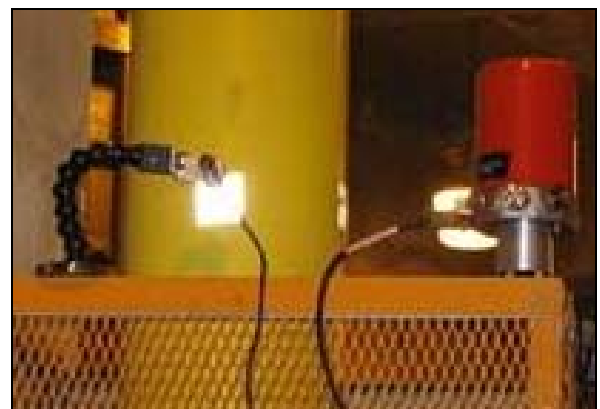
Figure 13. Laser Tachometer with Battery Powered Transmitter (Red) with Pulse Input for Pump Rotational Speed.
