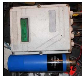
Figure 5. Ultrasonic Flow Meter With Loop Powered Transmitter.
