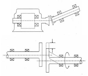
Figure 6. Illustration of Angular and Offset Misalignment
