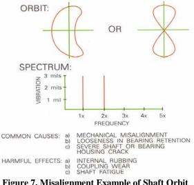
Figure 7. Misalignment Example of Shaft Orbit and FFT Spectrum
