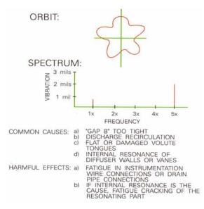
Figure 12. Vane Pass Vibration
