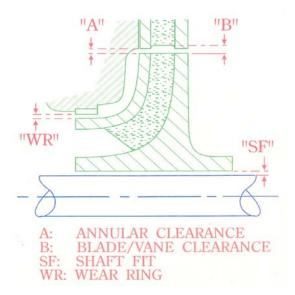
Figure 13. Various Impeller Gaps of Importance
