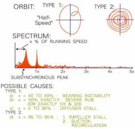
Figure 9. Subsynchronous Vibration
