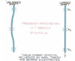
Figure 16. Vertical Pump Lineshaft Rotor Behavior
