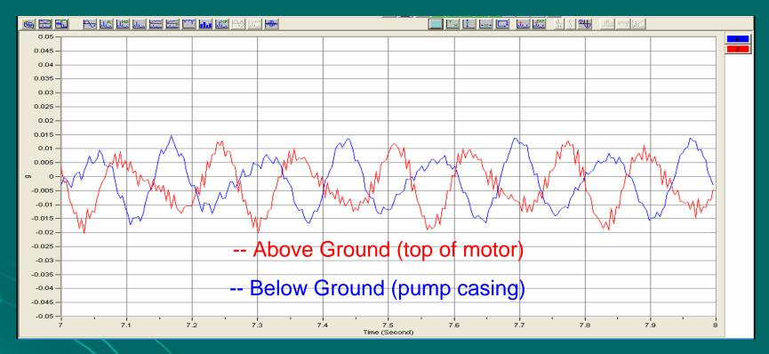
Traces indicate out-of-phase motion of top of motor compared to pump casing
