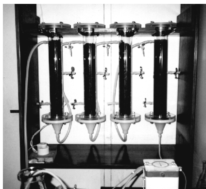
Figure 1. Continuous bioreactors used for the biosorption of \text{Cd}^{2+} , \text{Cu}^{2+} , \text{Zn}^{2+} and \text{Mn}^{2+}
