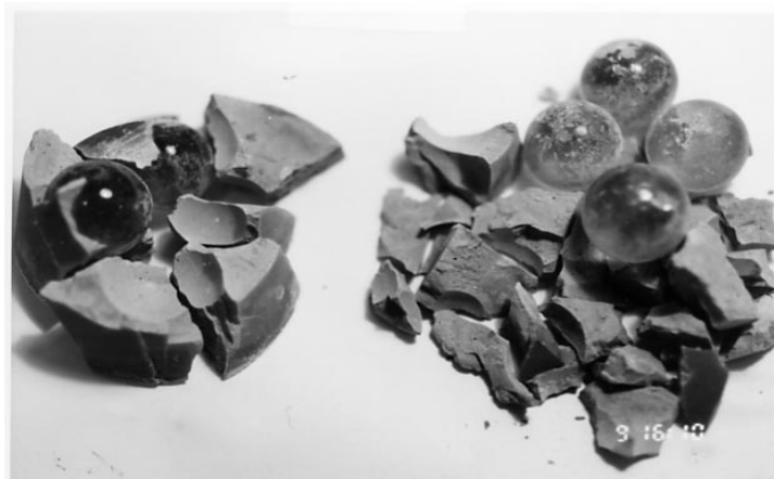
Figure 14. A photograph of concrete after electrical crushing
