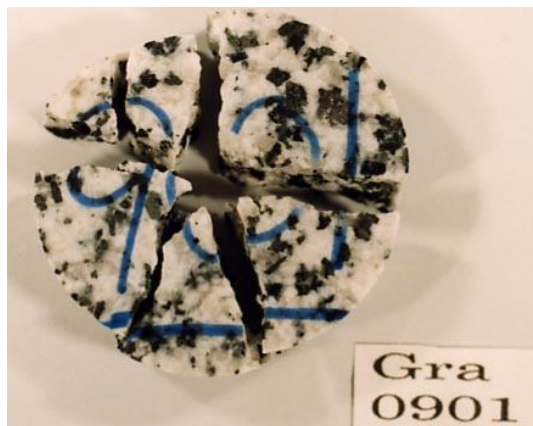
Figure 11. A photograph of a granite specimen after electrical crushing
