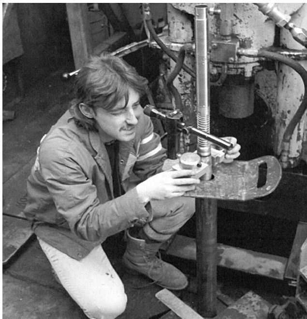
Figure 7: Gyroscope orientation is determined with respect to geographic north by sighting on known points.
