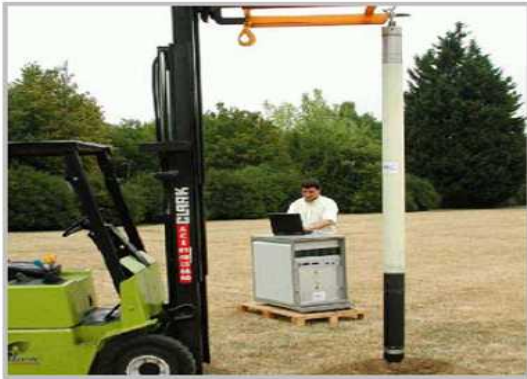
Figure 2: Neutron Activation. Prompt Gamma Neutron Activation multi-element assay system.
