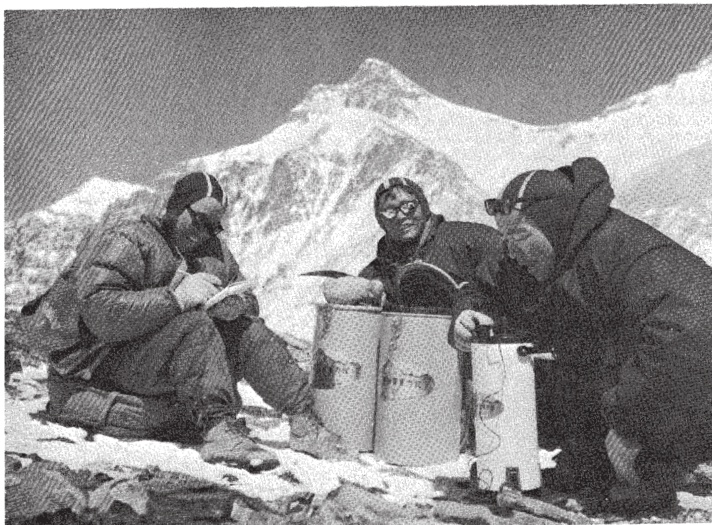
Figure 40.1. Chinese mountaineers making measurements with the "Mt. Jolmo Lungma" type gravimeter in the Mt. Jolmo Lungma region. (GSC 203492-D)
