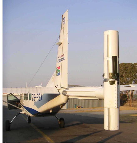
Figure 28: Exterior view of a cryogenic magnetometer mounted in a stinger on a fixed wing aircraft (Killeen, 2006).
