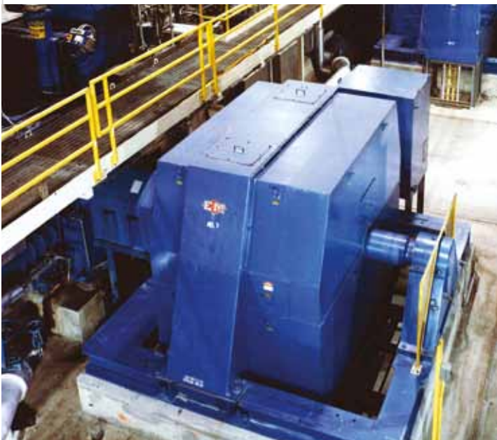
Synchronous motors 7000 HP at 327 RPM with TEWAC enclosures driving grinders at a paper mill.
