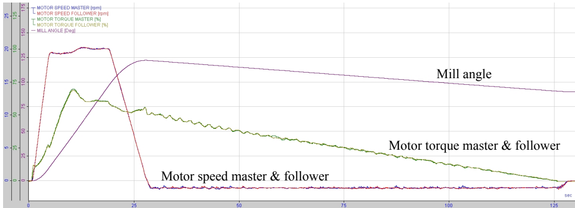
Figure 15: Automatic positioning routine with 90° angle reference (Copper Mountain SAG mill)
