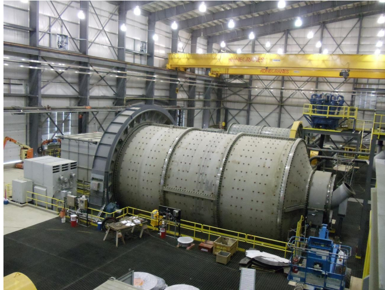
Figure 3 - The 24' x 39.5' ball mill
