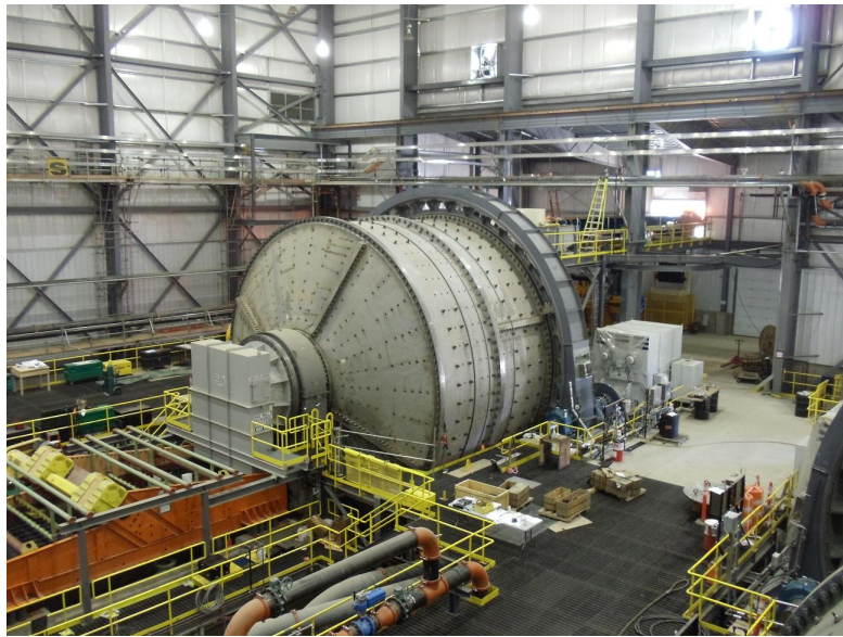
Figure 2 - The 34' x 20' SAG mill
