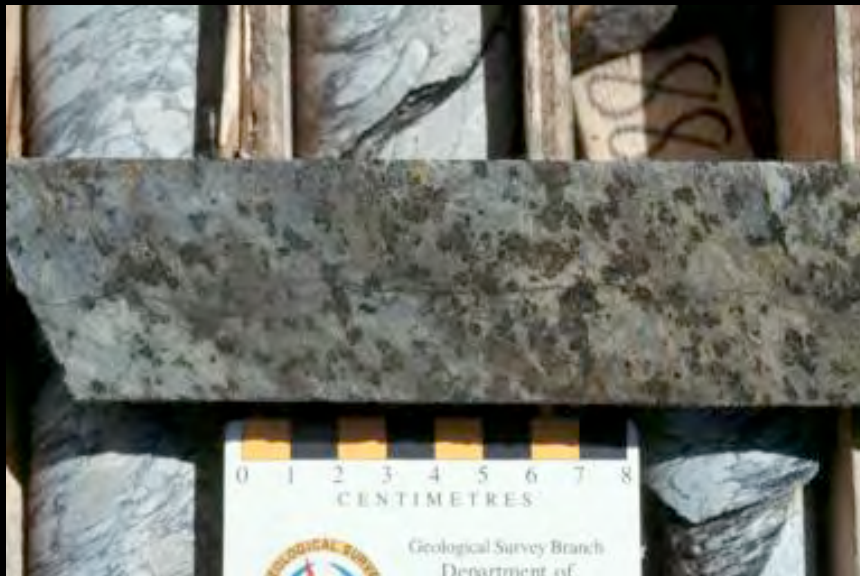
Chl-alt'd FW tuffs with chl clots ± Si alt'n (proximal)
