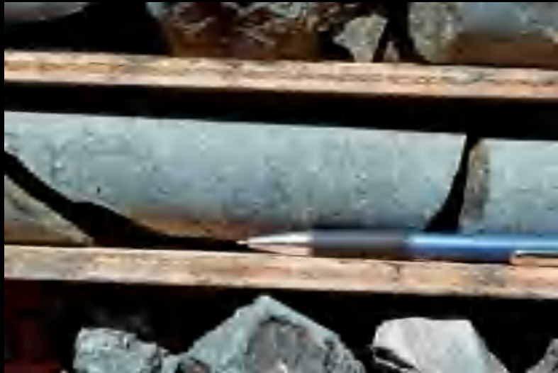
FW to sulfides— plag-phyrric basalt
