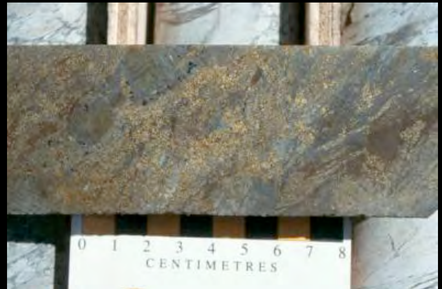
FW – chl-alt'd tuffs with cpy-rich sulphide (proximal)
