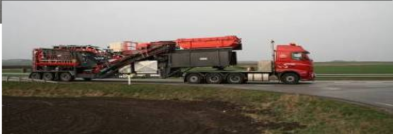
Rubber tire crushing & screening unit towed by fifth wheel
