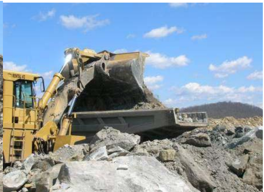
100 Ton Truck Loaded by a 15.7 yd 3 Wheel Loader
