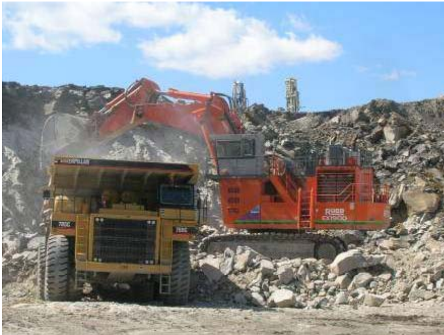
150 Ton Truck Loaded by a 15.7 yd 3 Hydraulic Excavator
