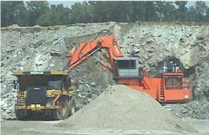
100 Ton Truck Loaded by a \text{yd}^3 Hydraulic Shovel
