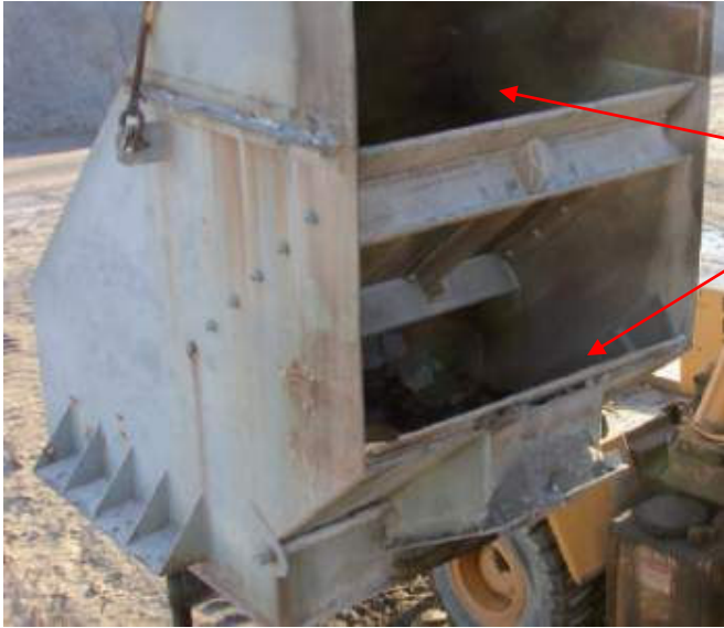
2 deck screen feeding to CS440
