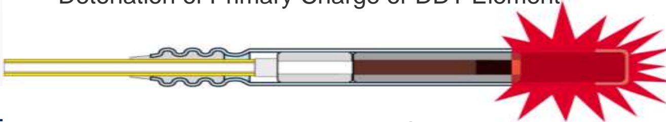
Detonation of Base Charge
