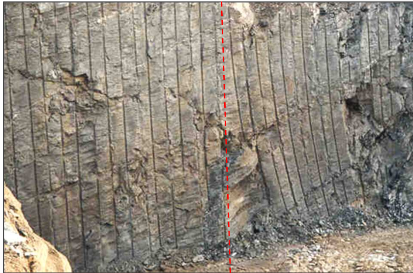
Deflection with and without pilot tube for Ø89 mm DC retrac bit / T51 in micaschist
