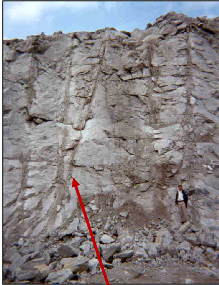
Directional error \text{Ø}3\frac{1}{2} " retrac bit / T45 in granite
