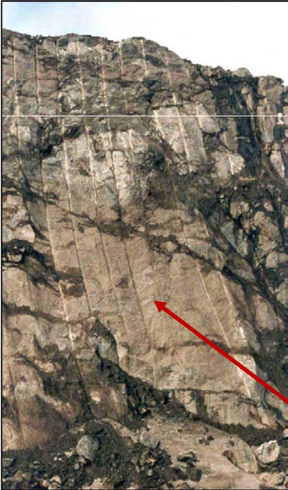
Deflection caused by gravitational sagging of drill steel in inclined holes in syenite
