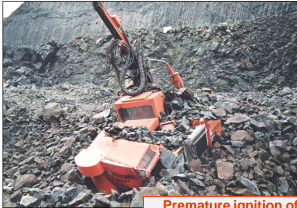
Premature ignition of electric detonators and blast due to lightning
