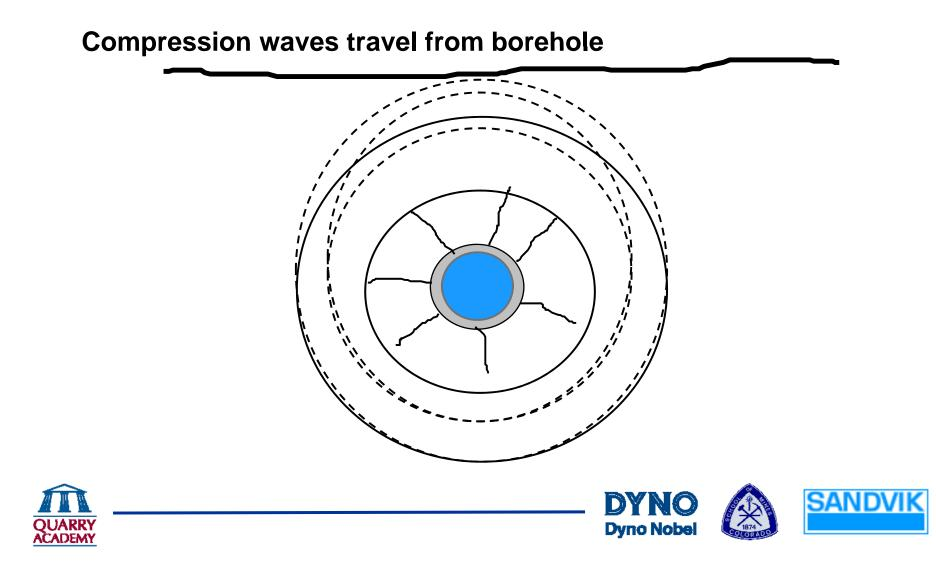
Compression waves leave the blasthole at firing time
