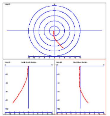
other. Specifically, hole three in the front row of holes shows deviation of six feet to the right and twelve feet to the front. Hole four in the front row showed deviation of seven feet to the left and twelve feet to the front.
