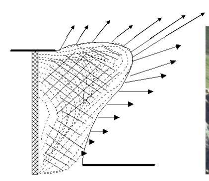
Inadequate Confinement Improper Face Movement
