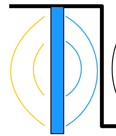
Compression waves travel to the open face, to the atmosphere and are reflected back into the mass as tension waves, pulling the rock apart
