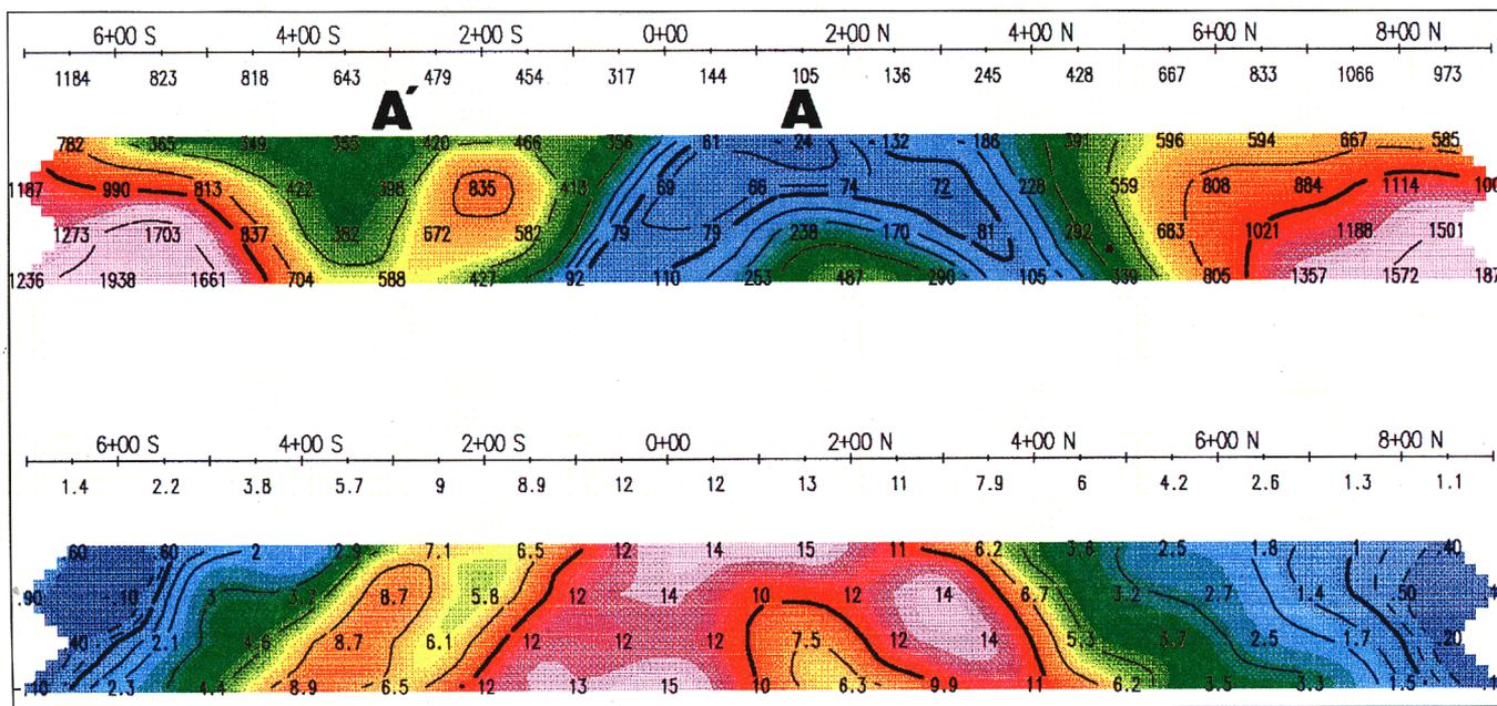
**Figure 9:** Pseudo-section of resistivity and induced polarization for line 800W, over the centre of the A zone (A). A' is a weak anomaly identifying minor sulphides but nevertheless is in ore and within the pit (Figure 7).
