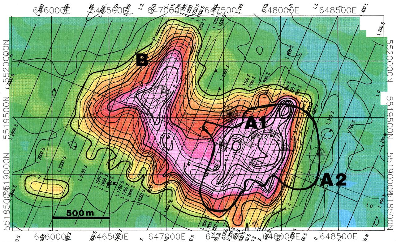
**Figure 7:** Induced polarization, contours of pant leg filter, from  $a=100$  m,  $n=1$  to 4, percent frequency effect, interval 0.5 PFE.
