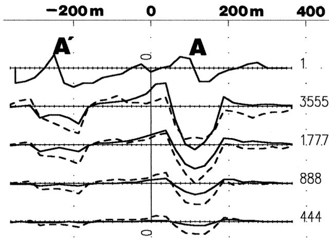
**Figure 12:** VLF-EM from Cutler, Mane, dip angle profile (1) on line 800 W, 1 cm = 20°. Horizontal loop MAXMIN EM profiles for frequencies 444 Hz to 3555 Hz, scale 1 cm = 40%. The largest anomalies rise to 40% of the primary field. Anomalies A and A' are the same as those on the resistivity section (Figure 9).
