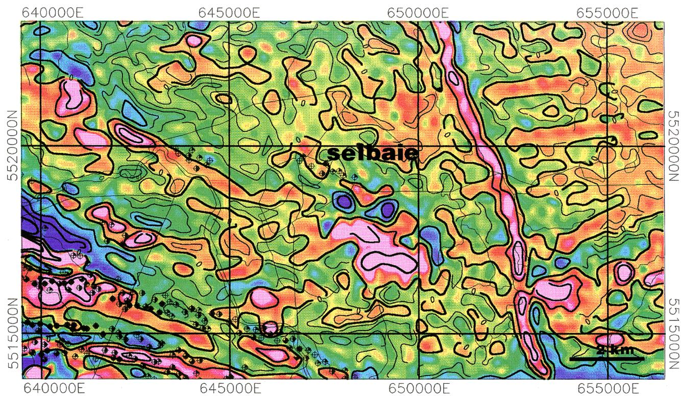
Figure 4: Contours of the first vertical derivative of the total magnetic field in Figure 3.
