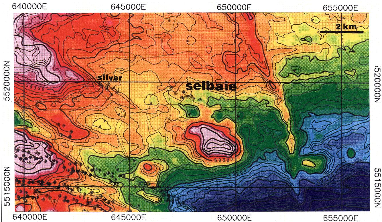
Figure 3: Contours of the total field magnetic response from the Brouillan-Manthet survey, minimum contour interval 10 nT.
