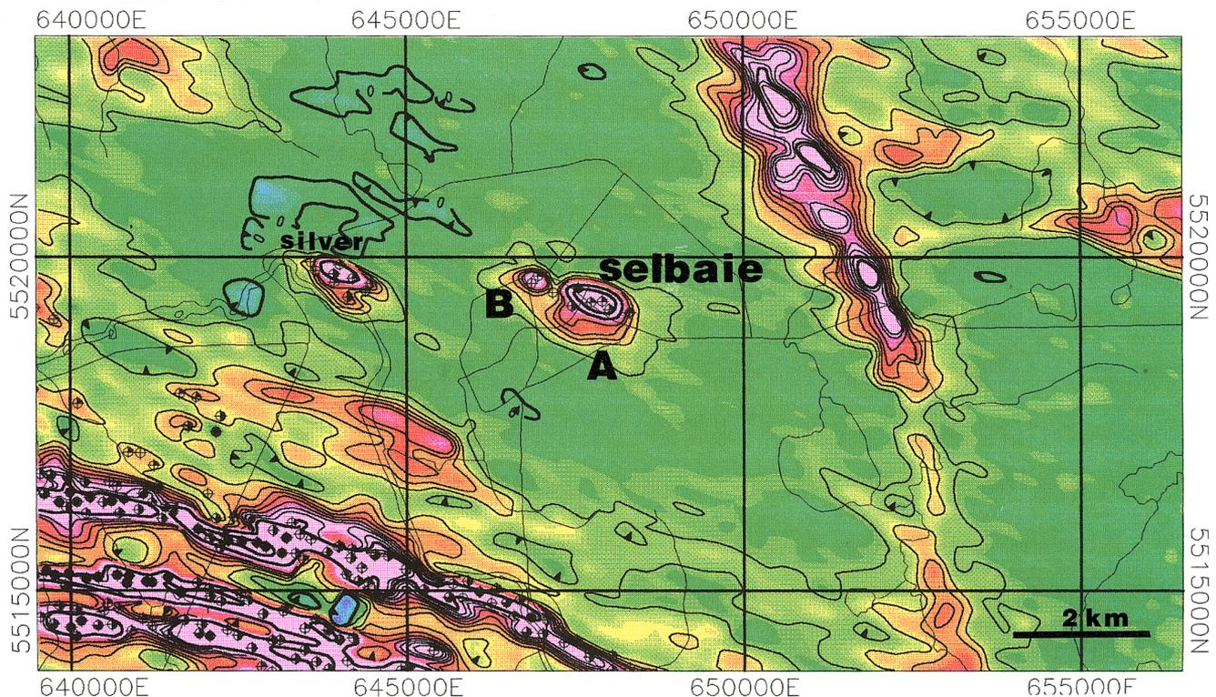
Figure 2: Contours of channel 1 of the Input airborne electromagnetic response with anomaly indicators, from the Brouillan-Manthet Input and magnetometer survey. The contour interval is 100 ppm of the primary field (ppm). The peak amplitude on the A zone is 3600 ppm, on the B zone 900 ppm.
