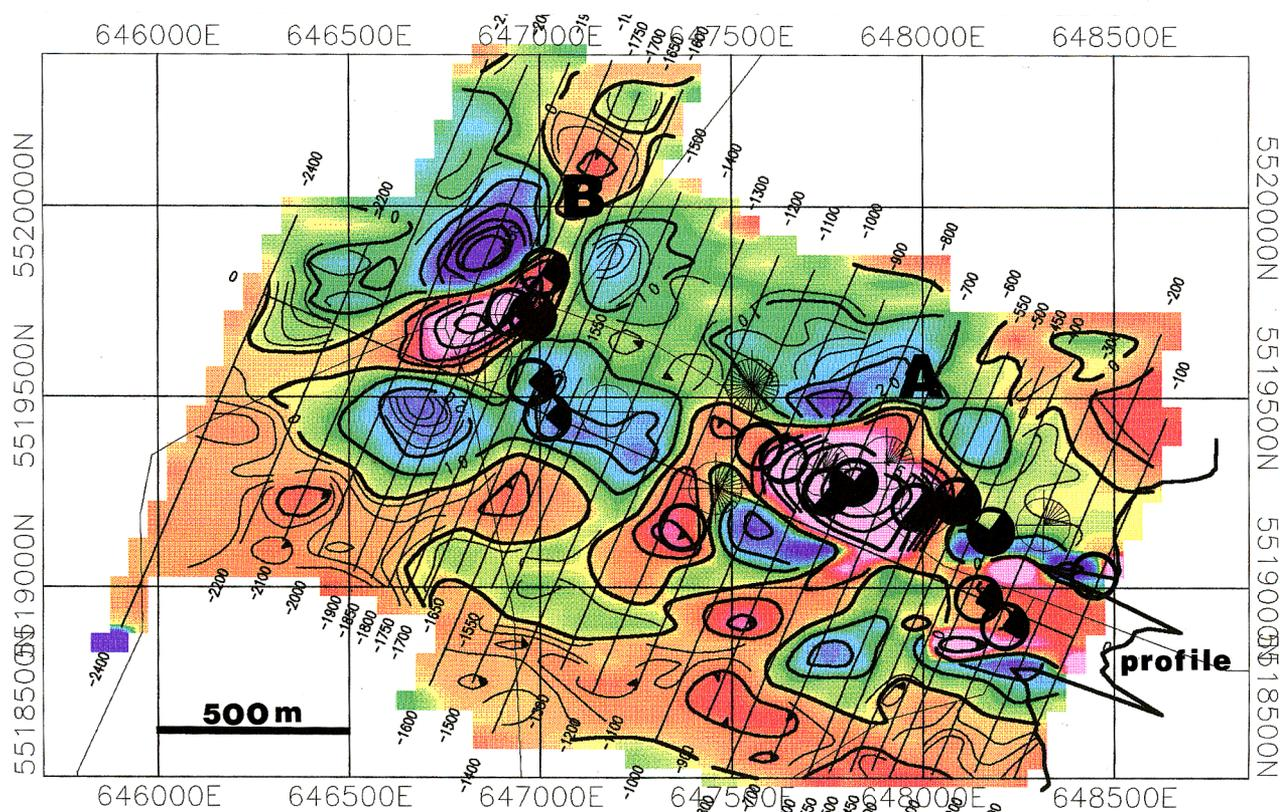
**Figure 10:** Contours of the in-phase horizontal loop EM response, 250 m coil separation. Peak amplitudes on the A zone are near -40% of the primary field. Anomaly indicators are from the 1971 Input survey. Less distinct are the anomaly indicators from the 1979 Input survey.
