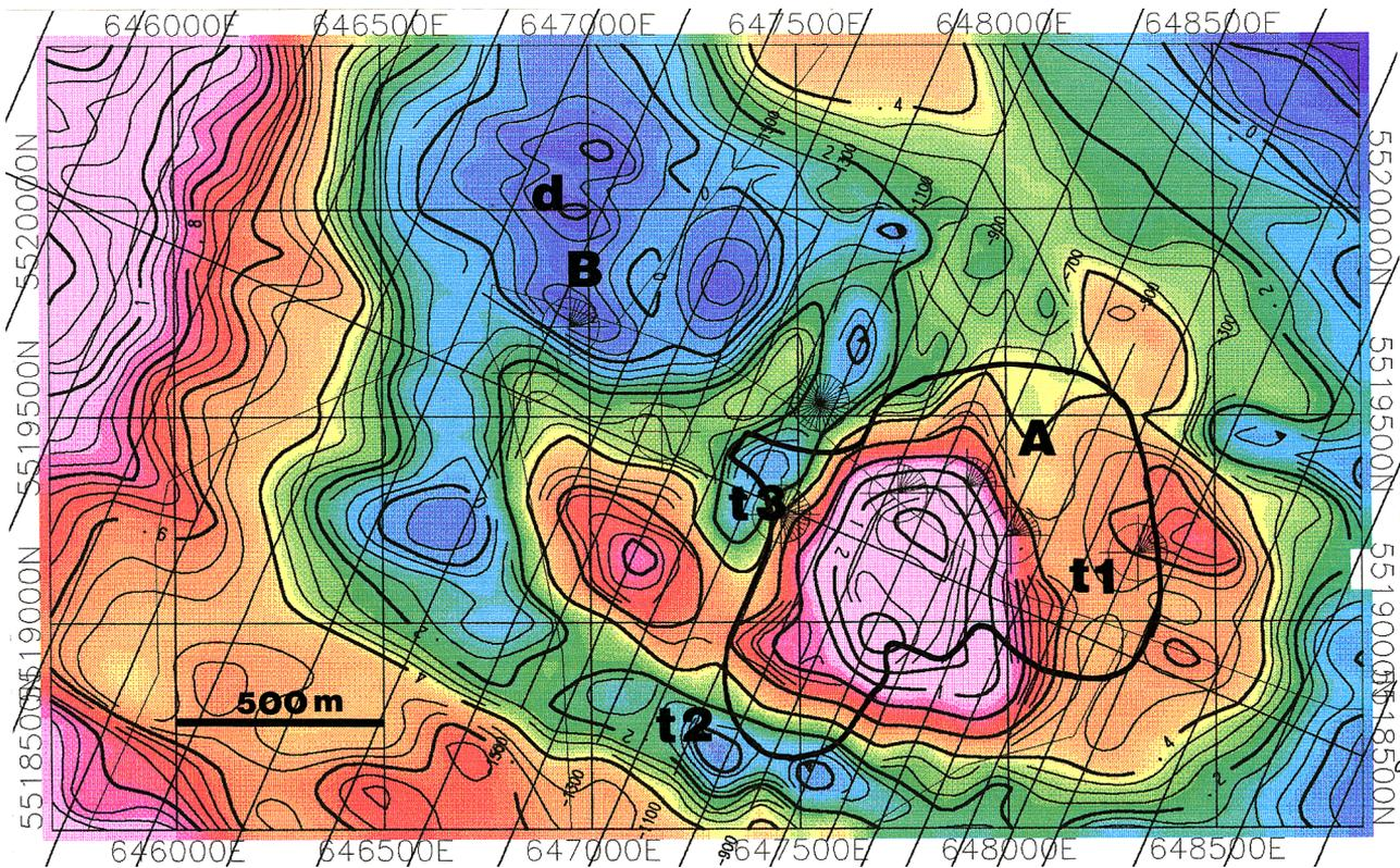
**Figure 13:** Contours of Bouguer gravity. The peak amplitude on the A zone is 1.4 mGal out of a local background of 0.2 mGal. t1, t2, t3 and d, are gravity lows caused by depressions in the bedrock surface. The land surface on which the gravity readings were taken was essentially flat, so that all bedrock surface irregularities were filled with low density overburden.
