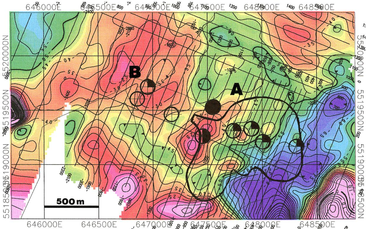
**Figure 6:** Ground total field magnetic field. Contour interval is 5 nT. Anomaly indicators are from the 1979 Brouillan-Manthet airborne Input survey. These are in the background for reference on the other ground maps as well as the airborne maps.
