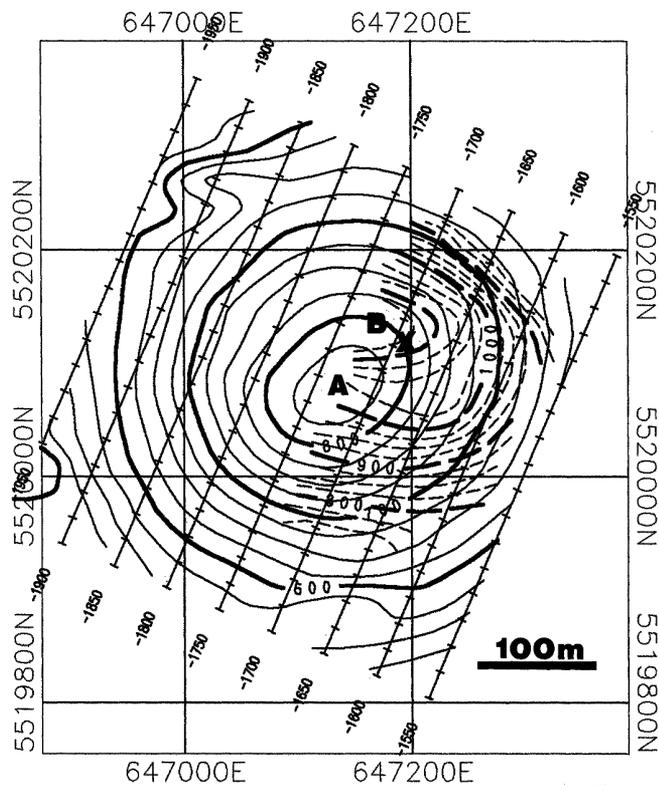
**Figure 14:** *Mise-à-la-masse* in the pipe-like feature at the north end of the B zone. The current source is in a drill hole at X, 300 m below the surface.
