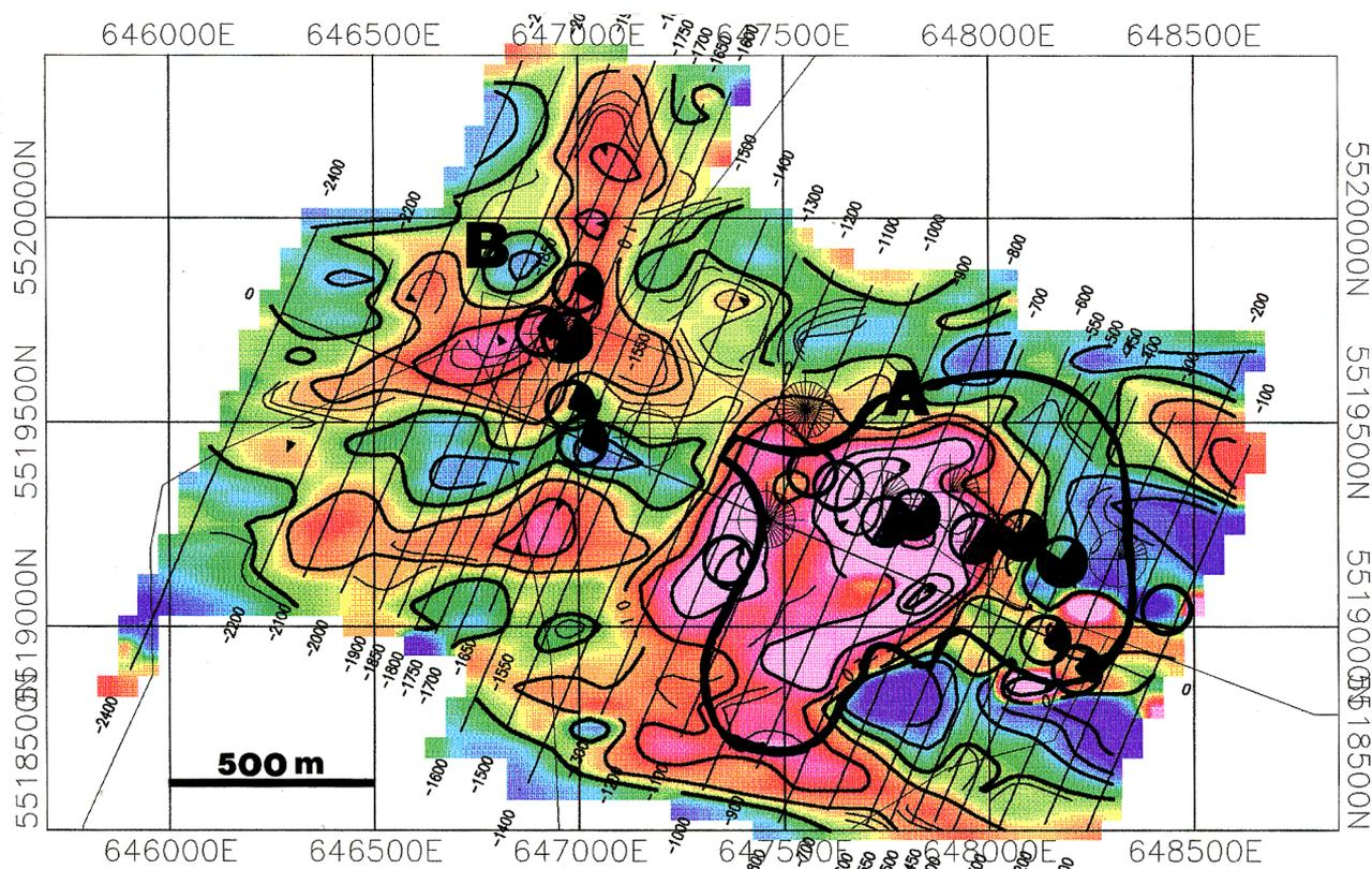
**Figure 11:** Contours of the quadrature horizontal loop EM response, 250 m coil separation. Peak amplitudes on the A zone are over -40% of the primary field. The quadrature response well describes the weaker mineralization in the southern extension of the A zone, and shows the narrow width and changes in strike of the B zone.
