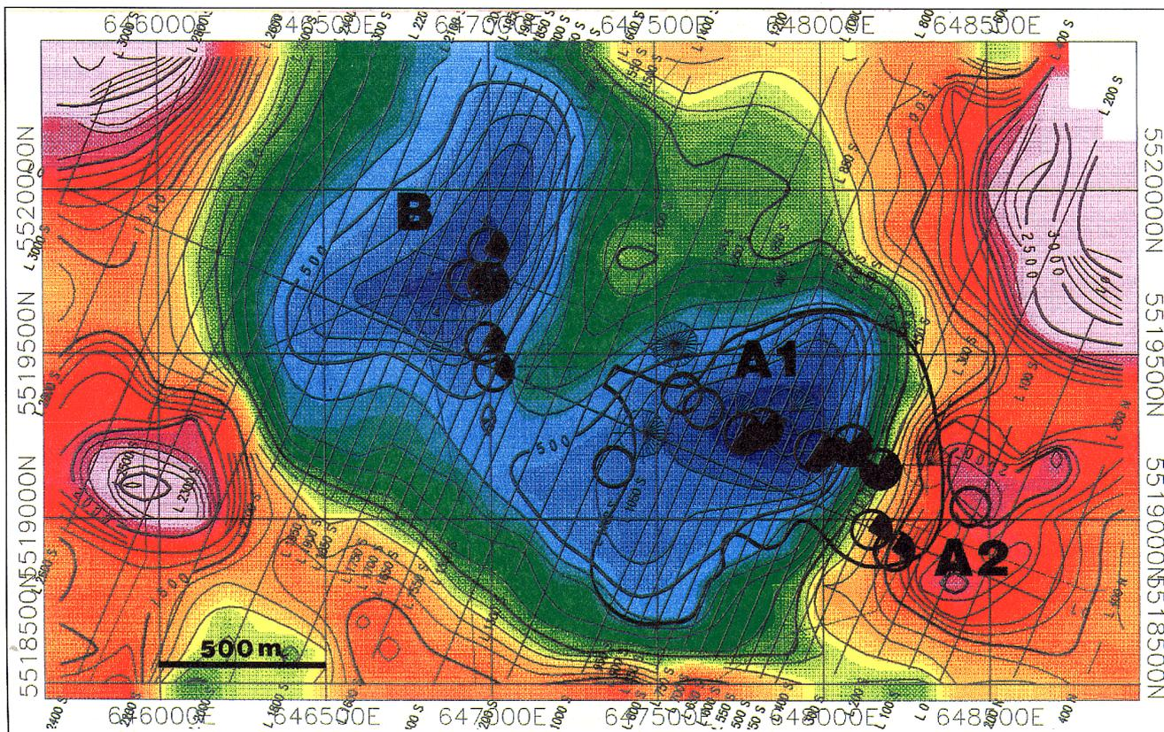
**Figure 8:** Resistivity, contours of pant leg filter, interval 100 ohm-m. Resistivities are below 200 ohm-m over the A1 and B zones. Anomaly indicators from the detail 1971 Input survey. Note that the A2 zone which has an upper lens with a top at 75 m from surface, is seen by the Input, but not by the resistivity or the IP. In section, the widest electrode spacings begin to see this deep zone.
