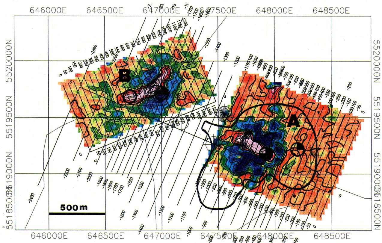
**Figure 5:** Contours of the Geonics EM 17, ground horizontal loop EM in-phase response. Anomaly indicators are from the 1971 discovery Input survey. Outline is of the 1996 pit, presented for reference on all the ground drawings.
