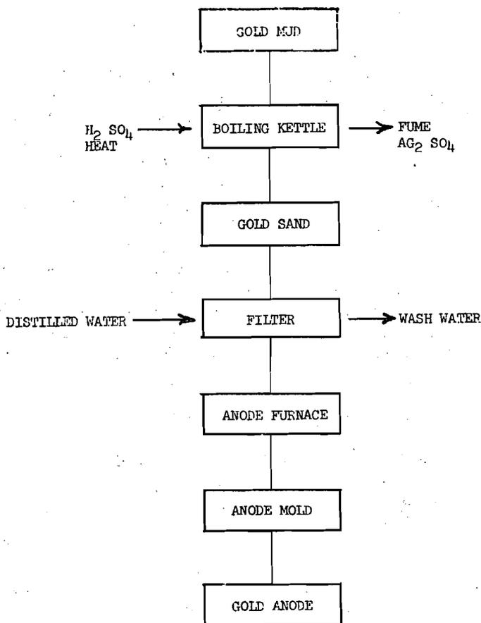
Figure 5. - Process Flow of Anode Mud to Gold Anode
