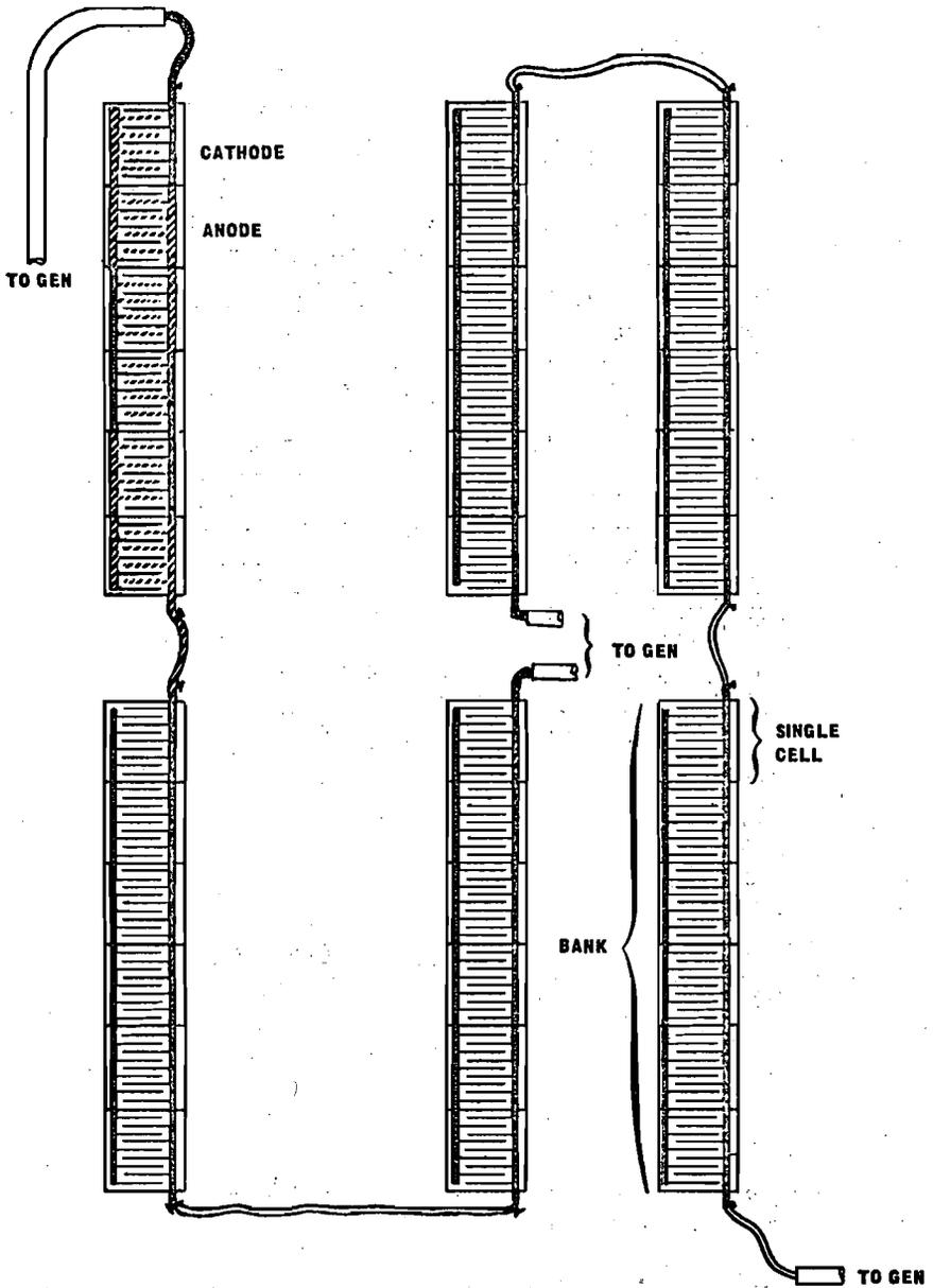
Figure 3. - Moebius Cell Banks Multiple Circuit
