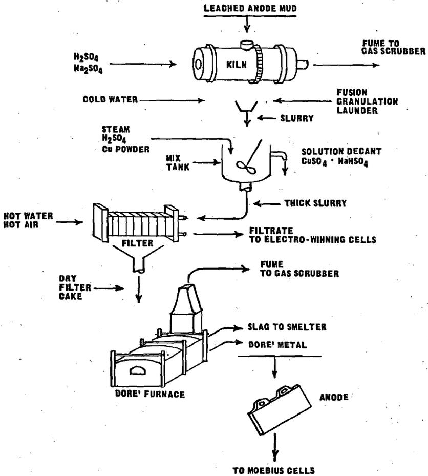
Figure 1. - Simplified Flow Sheet for the Treatment of Anode Slime
