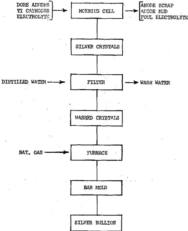
Figure 2. - Summary Flow Sheet for the Parting of Dore' Metal
