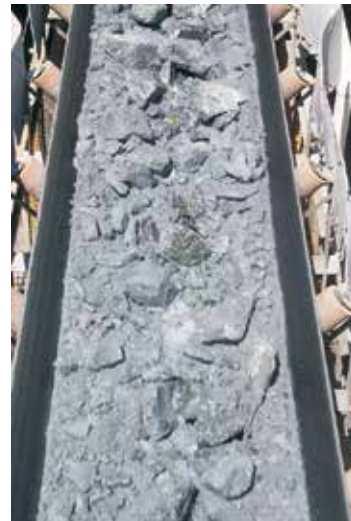
FIG 4 - View of muck on a conveyor.
