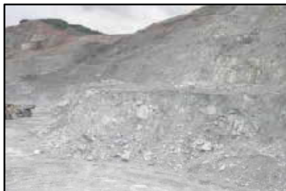
FIG 20 - Model validation against actual pit blast . The photograph in the bottom right indicates the tight muckpile with coarse fragmentation resulting from insufficient blast energy.
