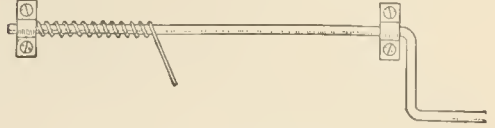
A Copper Wire Wrapped around and Soldered to a Straight Rod for a Lead Screw
