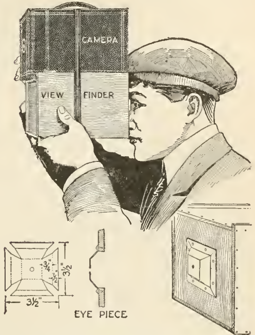
Sight through the Eyepiece for a Direct View of the Object Photographed, Thus Insuring More Nearly the Accuracy of the Result
