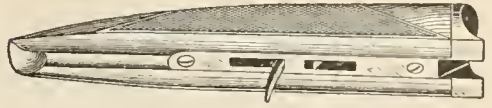
The Fore End Is an Extension of the Stock beyond the Triggers and the Frame
