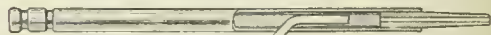
Blowpipe Connection to the Ordinary Illuminating-Gas Main for Hard and Soft Soldering
