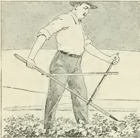
Much of the Tiring Labor in Using a Hoe or Rake is Overcome by This Simple Homemade Attachment
