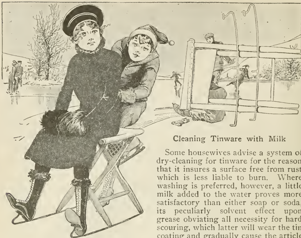
A Camp Chair Constitutes the Body of the Sled and the Legs are Equipped with Runners
