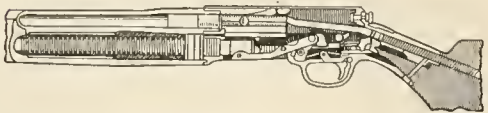
A Self-Loading Shotgun in the Positions of the Action Open and Closed
