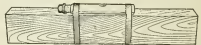
A Bottle Filled with Water and Tied to a Straight Piece of Wood for a Level
