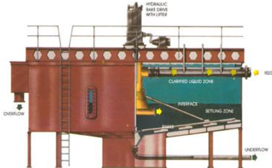
Figure 3: A counter current decanter thickener tank showing how liquid and the settled solid are separated (Gold metallurgy, 2011).
