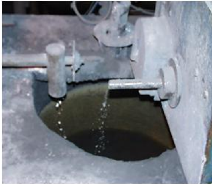
Figure 9: Addition of zinc and lead nitrate (Gold Metallurgy, 2011)
