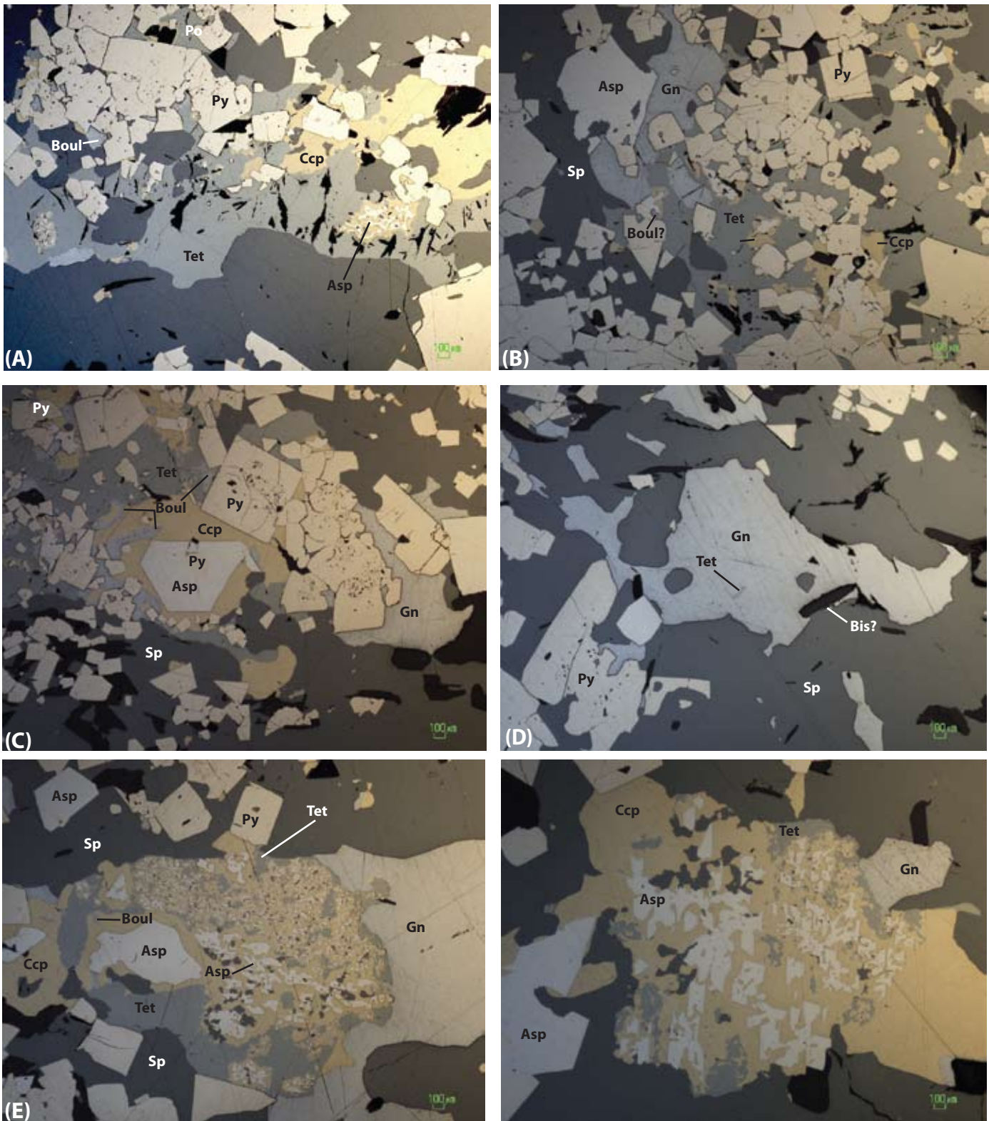
Figure 5. Sample 36505. A) Tetrahedrite-sphalerite-pyrite-chalcopyrite-bearing assemblage with chalcopyrite-arsenopyrite-tetrahedrite intergrowths in tetrahedrite. Note the polishing cleavage in the tetrahedrite. B) Pyrite-galena-tetrahedrite-arsenopyrite-chalcopyrite-boulangerite(?) assemblage. C) Euhedral pyrite and arsenopyrite grains with chalcopyrite, tetrahedrite, galena, sphalerite, and boulangierite. D) Pyrite and sphalerite with galena that has inclusions of tetrahedrite (exsolution blebs) and potential bismuthinite. E) Intergrowths of tetrahedrite-arsenopyrite needles-chalcopyrite within tetrahedrite and galena with arsenopyrite, sphalerite, and pyrite nearby. F) Close up of a chalcopyrite-tetrahedrite-arsenopyrite intergrowth with galena, sphalerite, pyrite, and larger arsenopyrite grains nearby. These intergrowths commonly host gold in the 1806 zone.
