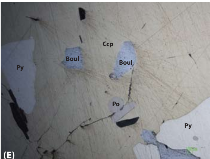
Figure 21. Sample 36521. A) Sphalerite-pyrite-chalcopyrite-porrhrotite-bearing sulfides with hematite associated with gangue phases. B) Pyrite-pyrrhotite-sphalerite-chalcopyrite-sulfides. C) Pyrite-pyrrhotite-galena-sphalerite-chalcopyrite-bearing sulfides. Note multiple growth zones in pyrite mass. D) Pyrrhotite with inclusion of arsenopyrite and sphalerite-chalcopyrite. E) Chalcopyrite with inclusions of boulangerite, euhedral pyrite, and pyrrhotite.
