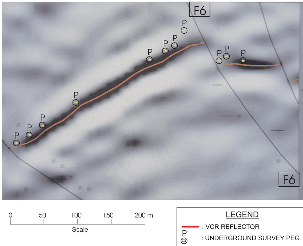
Figure 10: Mining confirmation of VCR seismic structure plan at Vaal Reefs No. 10 Shaft.
