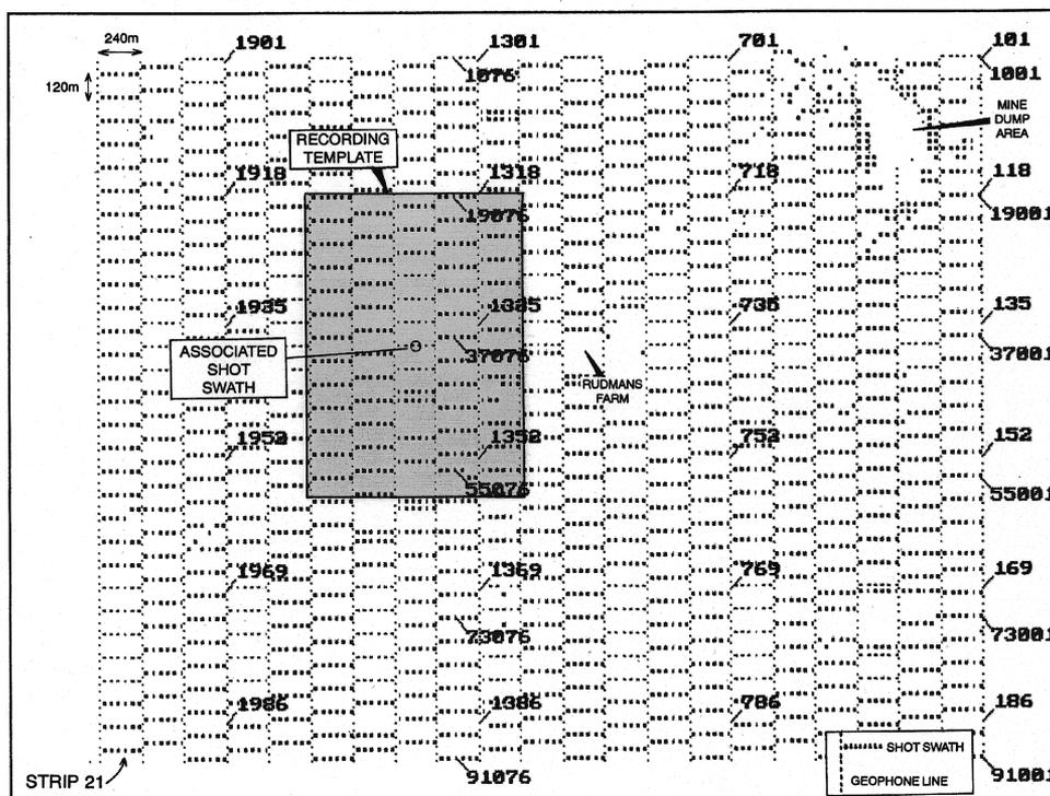
Figure 6: Acquisition geometry employed at Vaal Reefs No. 10 Shaft.
