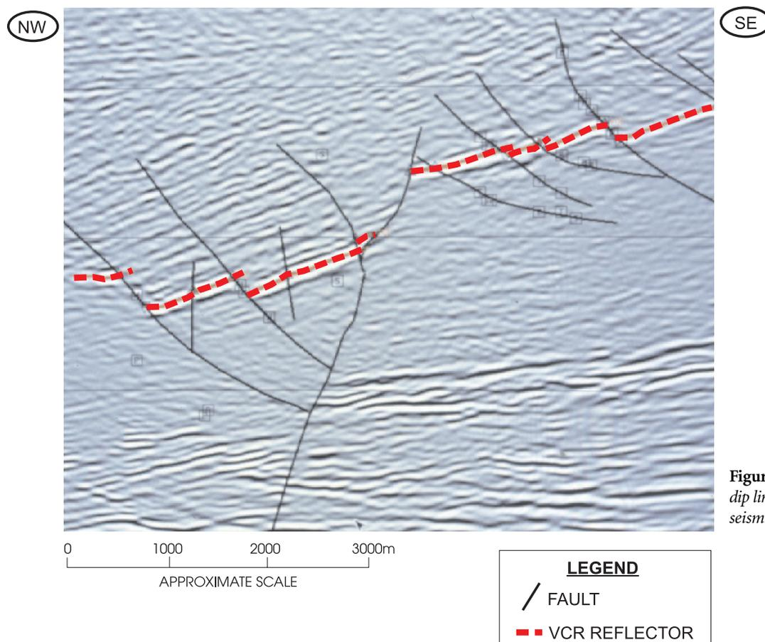
**Figure 7:** Portion of an interpreted dip line through the center of the 3-D seismic data cube.
