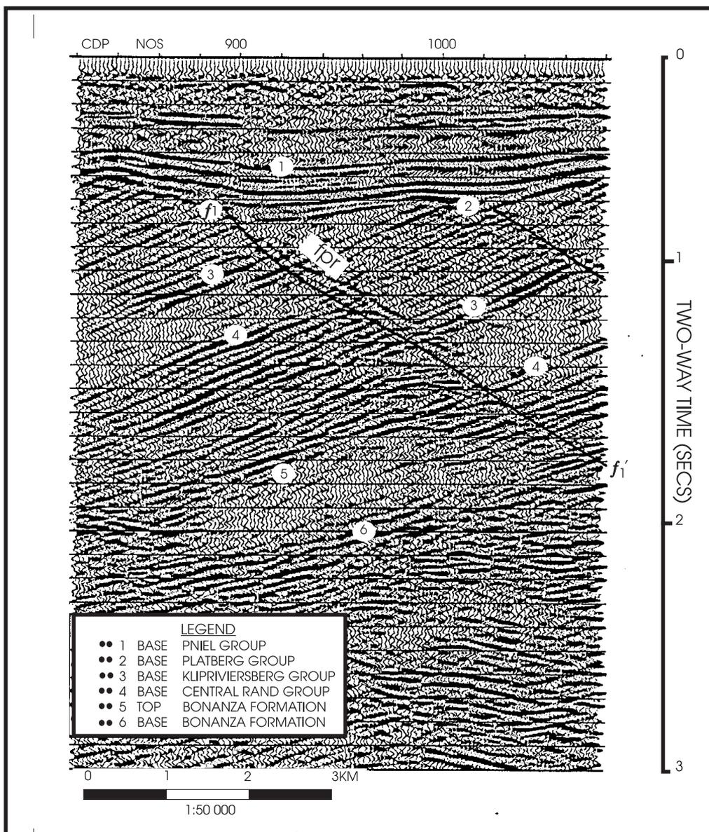
Figure 4: A portion of 2-D seismic line OG-54 in the vicinity of 10 Shaft.
