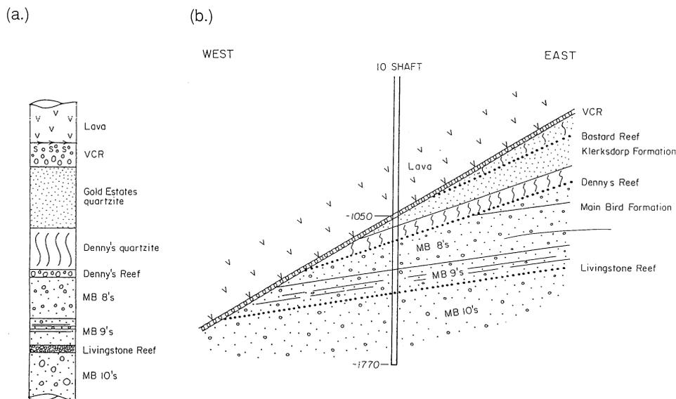
Figure 3: (a) Generalized geological section No. 10 shaft. (b) Idealized west-east section across the No. 10 Shaft Lease Area showing unconformable relationships. (Ref: Trewick (1994))
